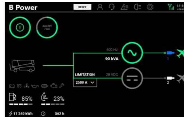
DDM 090 Control Panel Screen
